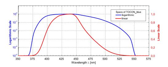
GaP blue light detector with integrated amplifier
